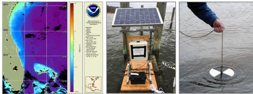
Figure 5. Variety of methods employed by QSI for measuring and monitoring turbidity – MODIS kd490 (left), turbidity meter (middle), and Secchi disk (right).
